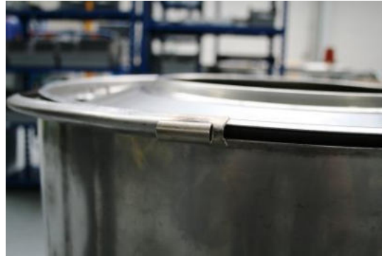
Outer tub seal
