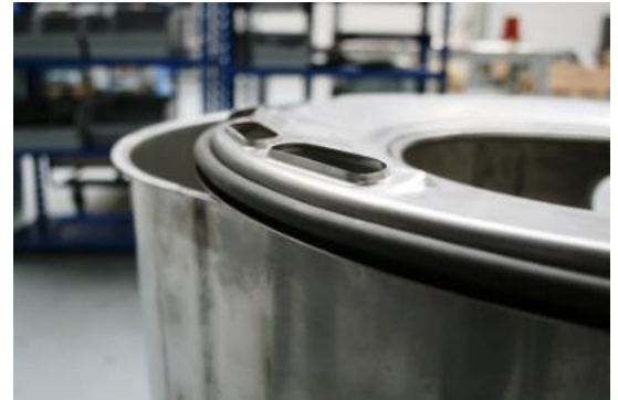
Outer tub seal
